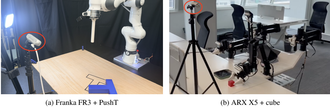
Figure 8: Real-robot setups (red circle: single third-person RGB camera) . Both platforms use a single tripod-mounted RealSense camera as the only RGB sensor feeding the planner; no wrist or egocentric cameras are used. (a) Franka FR3 with a RealSense D455 viewing a wooden tabletop; the blue T-block must be aligned with the marked target outline. (b) ARX X5 on an Agilex Mobile ALOHA with a RealSense D435i viewing an office desk; the arm transports a single red cube.
